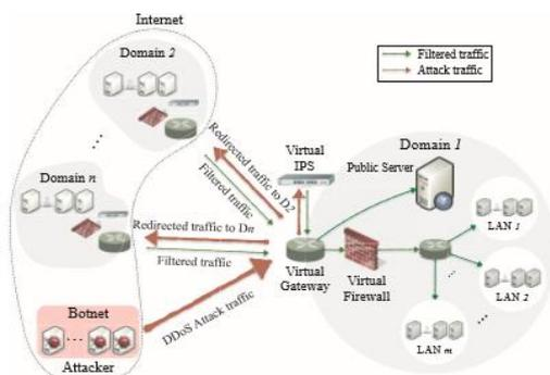
Figure 1 CoFence Diagram
