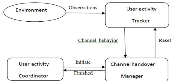
Fig 3. Channel Handover Procedure
