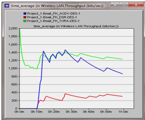
Fig 15: Throughput in Frequency Hopping
