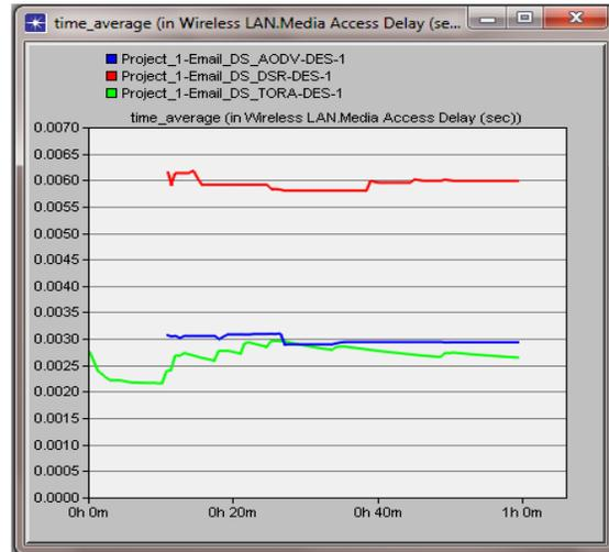
Fig 6: Media Access Delay in Direct Sequence
