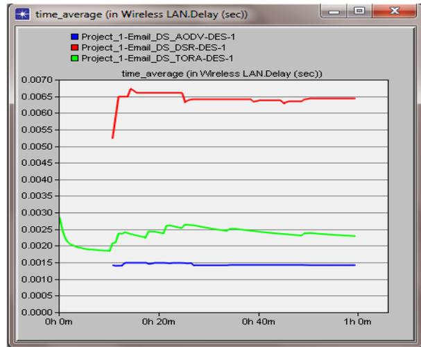
Fig 2: Delay in Direct Sequence
