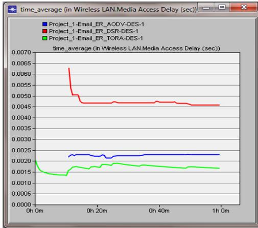
Fig 9: Media Access Delay in Extended Rate
