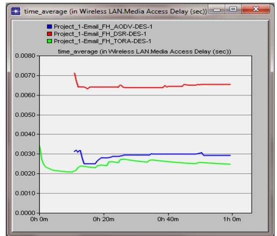
Fig 7: Media Access Delay in Frequency Hopping
