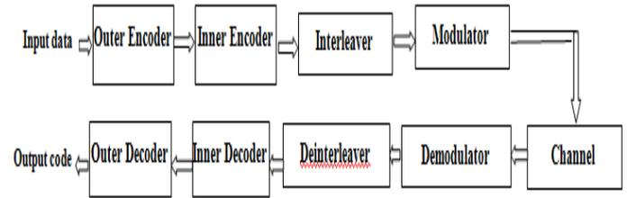
Fig. 11 Construction of Interleaved Concatenated Code
