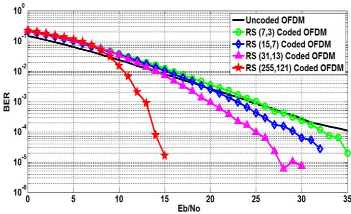
Fig. 6 Different Lengths RS Codes through Fading Channel
