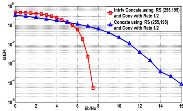
Fig. 136 Concatenated Coded System with and without Interleaver
