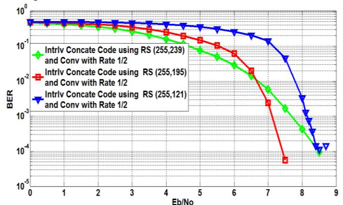
Fig. 12 Interleaved Concatenated Coded OFDM System
