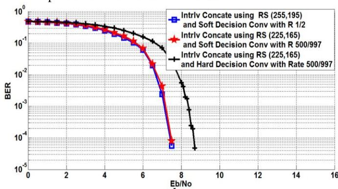
Fig. 147 Concatenated Coded OFDM with Shortened RS and Punctured Convolutional Codes
