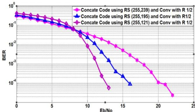
Fig. 103 Concatenated Coded OFDM System Performance
