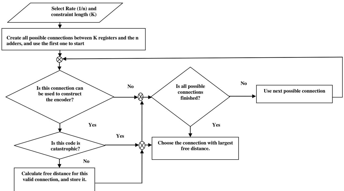
Fig. 11 An Algorithm to Select Convolutional Code with Large Distance
