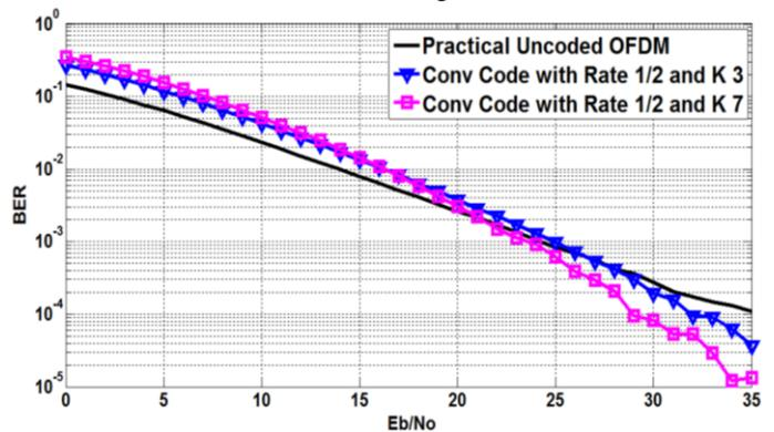
Fig. 8 Convolutional Coded OFDM
