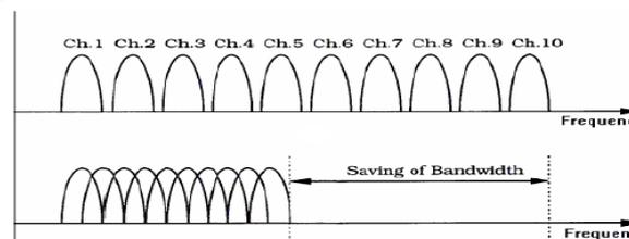
Fig. 1 Saving Bandwidth using OFDM
