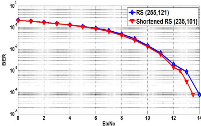
Fig. 7 Shortened RS Coded System
