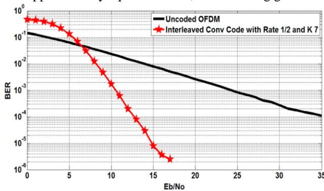
Fig. 8 The Interleaved Convolutional Coded OFDM
