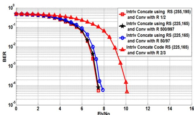
Fig. 1815 Concatenated Coded System with Different Rate Convolutional
