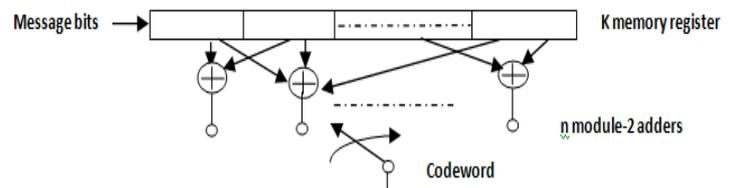
Fig. 3 Convolutional Encoder
