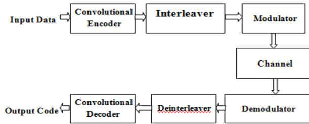
Fig. 9 Interleaved Convolutional Coded OFDM System
