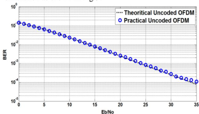
Fig. 5 Theoretical and Practical Uncoded OFDM
