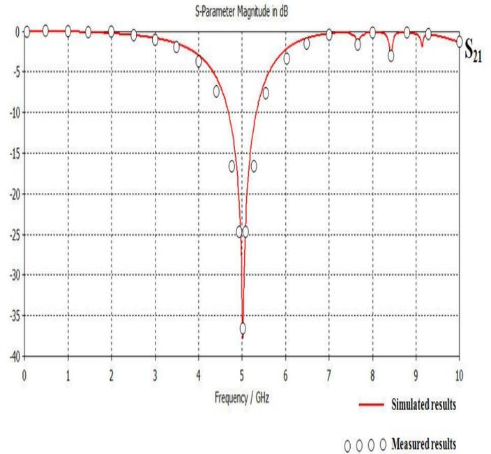
Fig. 7 Transmission characteristic curve for the proposed FSS structure in fig 6 showing the comparison of the simulated and the measured results with good transmission outside the intended band.
