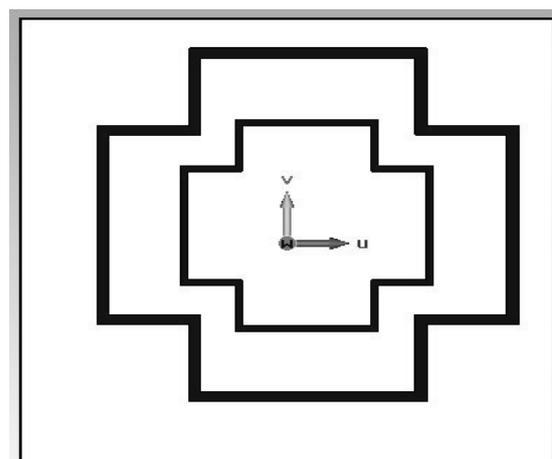
Fig. 4 Double stepped square structure that is placed on either side of the substrate.
