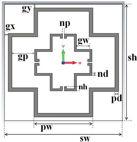
Fig. 6 the proposed unit cell FSS structure.
