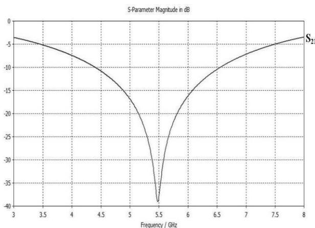
Fig. 5 Transmission characteristic curve for the L shaped structure symmetrically placed on all quadrants in combination with stepped square patch.
