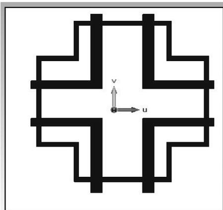
Fig.3 Stepped square patch in combination with an L shaped structure symmetrically placed on all quadrants of the unit cell.
