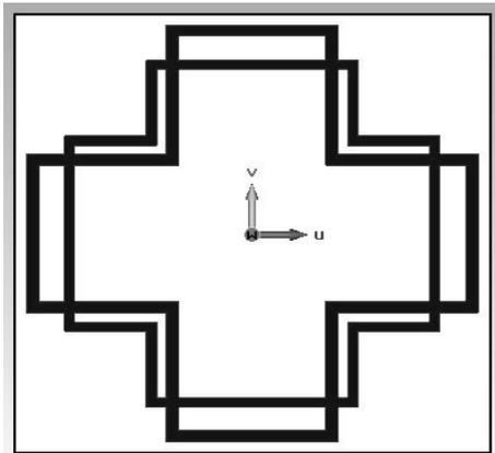
Fig.2 Modified double layers of stepped square patch on both sides of the substrate.
