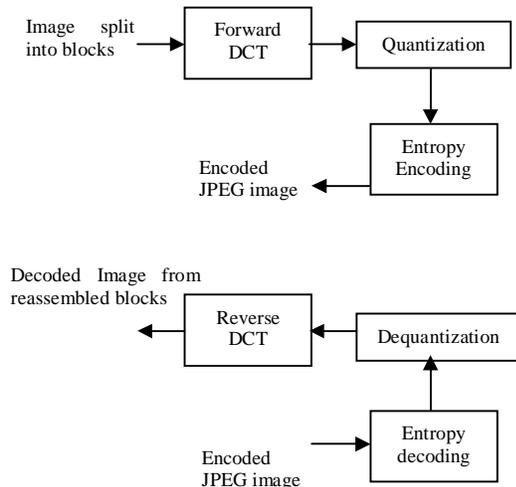
Figure 3. JPEG Encoding and Decoding
