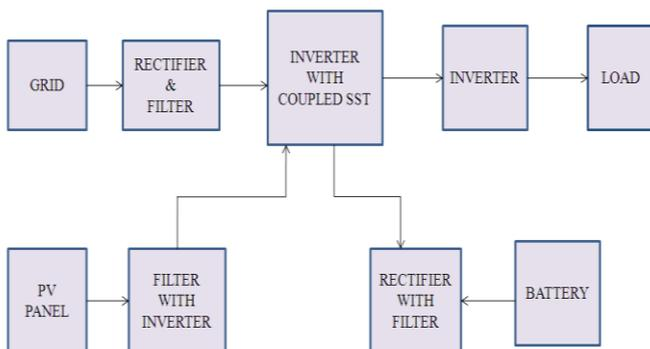
Fig.2. Block diagram for the proposed scheme
