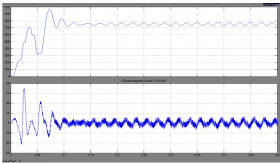
Fig.8. Speed & Torque Output Waveform
