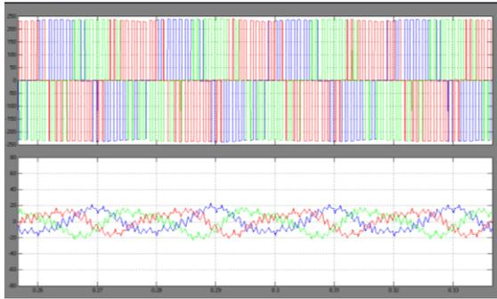
Fig.7 Voltage and current Waveform
