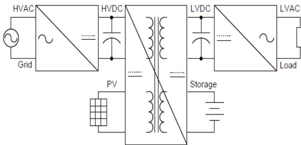
Fig.1. QAB-based SST with storage and PV
