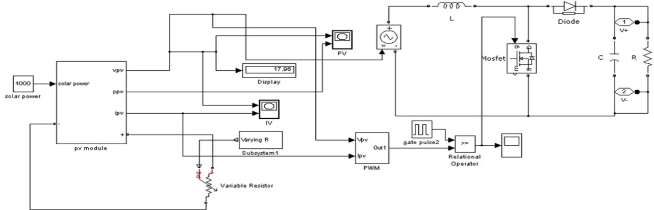
Fig.4. Simulink Model of proposed solar module
