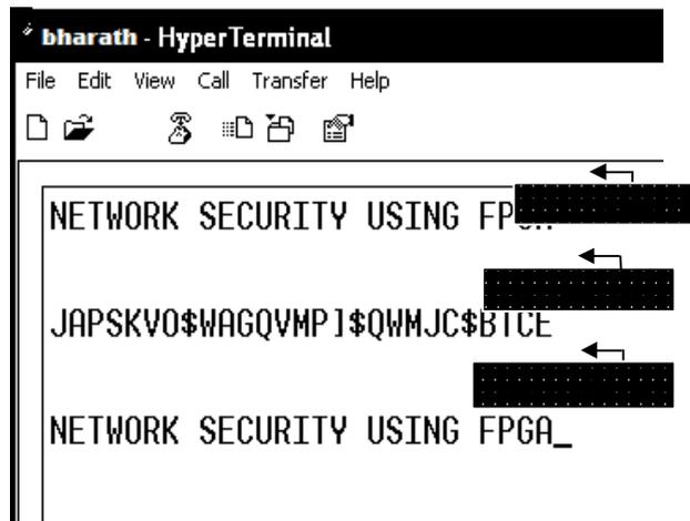
The above figure shows the output of Xilinx Spartan 3E FPGA device. At first the input fed to the FPGA device under normal mode. Then, the same input can be given under encryption mode to get encrypted data. This encrypted data can be saved in note pad to transmit to the receiver side. Now, the encrypted data can be given under decryption mode in the receiver side to get original data.
