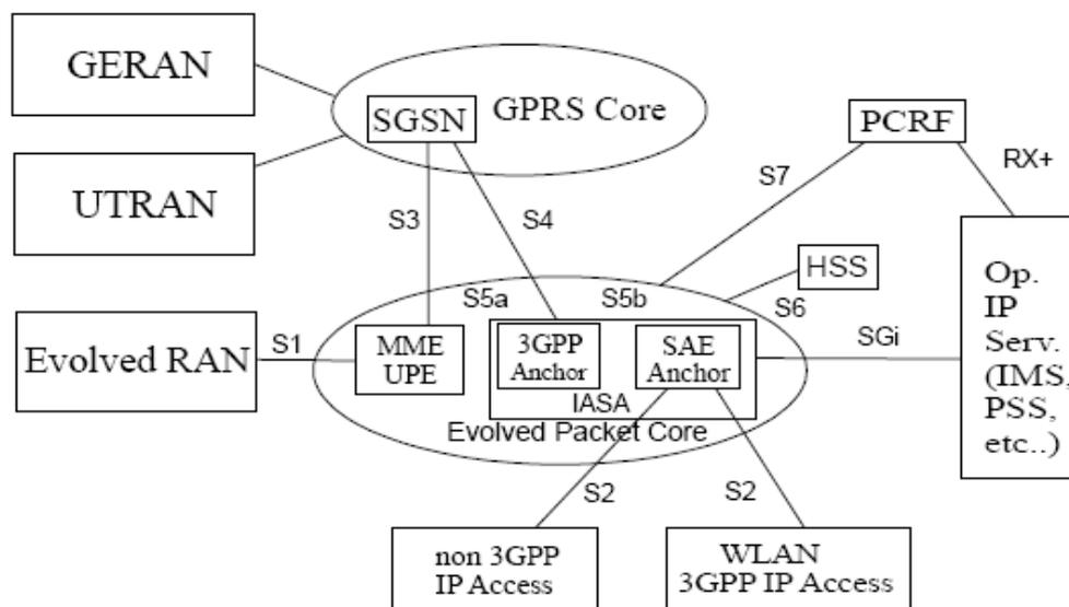
Fig. 2 LTE-SAE Architecture
