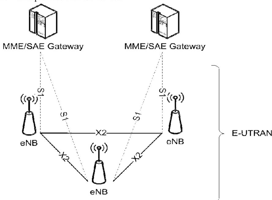
Fig.1 LTE architecture with E-UTRAN
